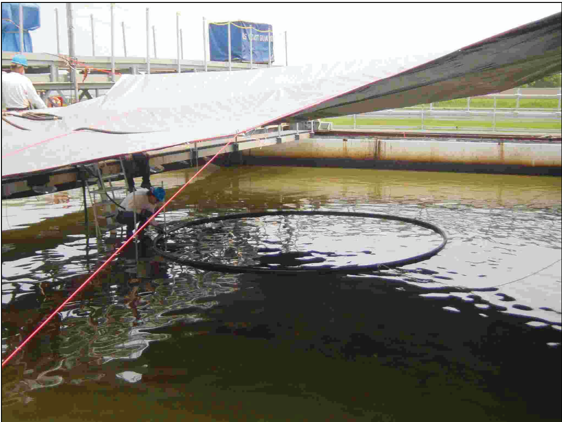
Figure 1 Ohmsett tank set up showing 4.6 meter diameter ring to contain oil under tarpaulin
