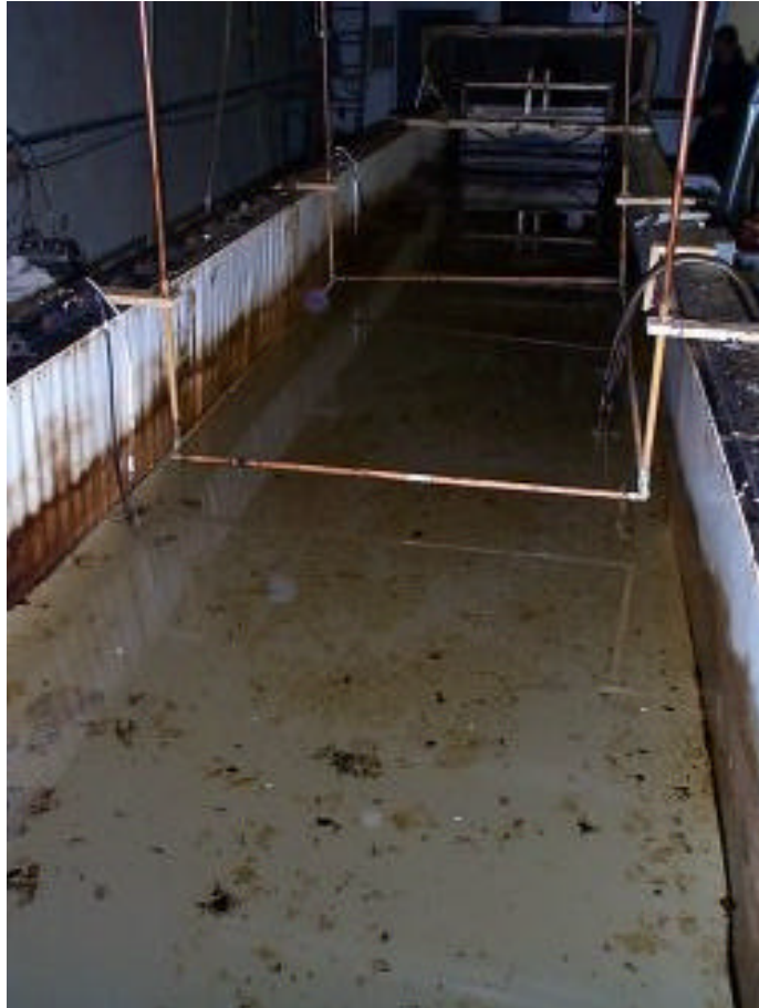
Figure 2: Air Bubble Curtain Piping
