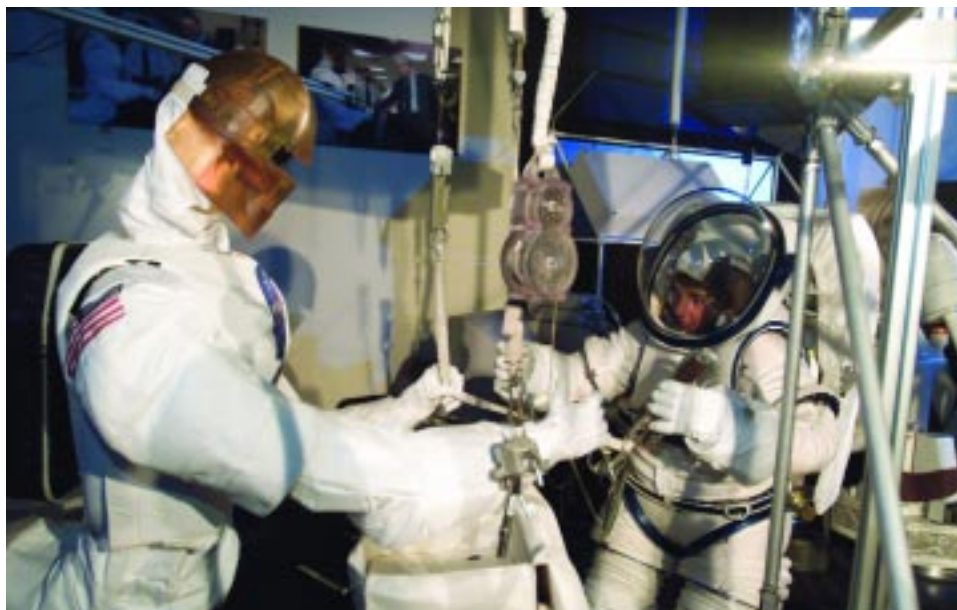
Figure 139: Astronaut Nancy Currie participates in a test with the Robonaut to evaluate human-robotic operations. The Robonaut is just one example of the types of robotic systems that will work alongside human explorers during future space missions.
