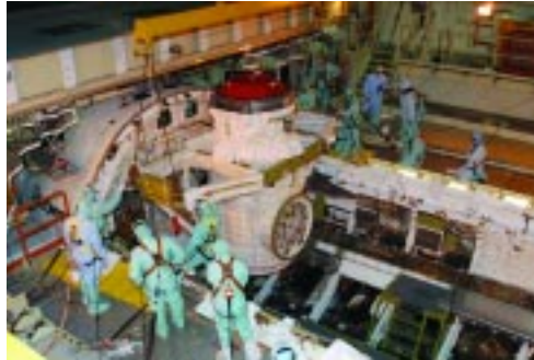
Figure 127: Crews help guide an airlock, hanging from a boom in the Orbiter Processing Facility at Kennedy Space Center, into Discovery's bay on May 12, 2004. All three Shuttles have undergone extensive maintenance and safety upgrades to prepare them for return to flight.
