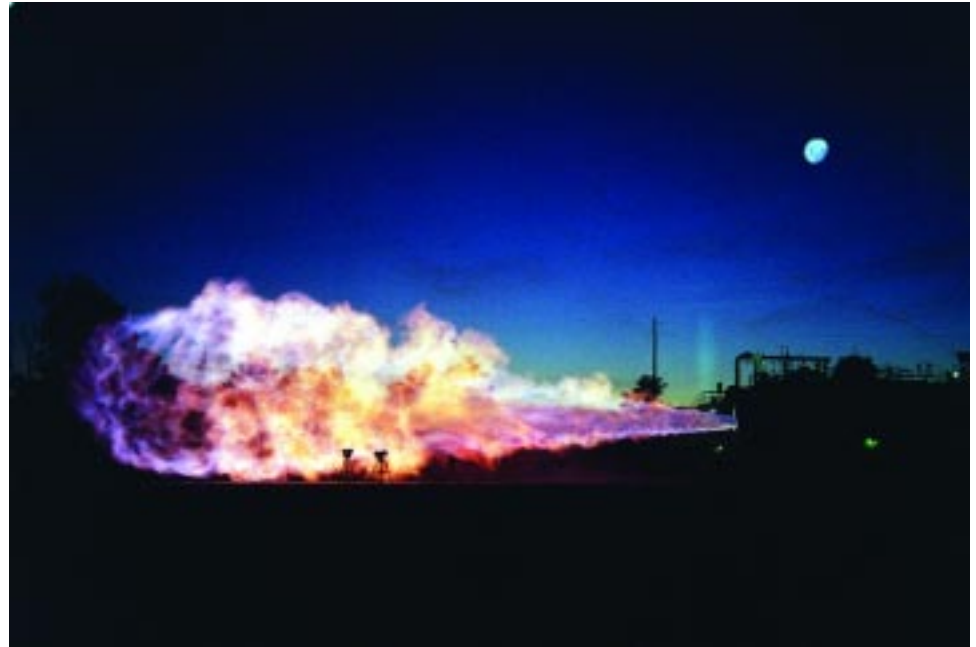
Figure 131: A 750,000 pound-thrust rocket engine undergoes a test firing at Marshall Space Flight Center.
