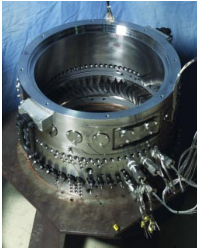
Figure 76: NASA's new two-stage, highly-loaded compressor casing assembly should improve engine efficiency.
