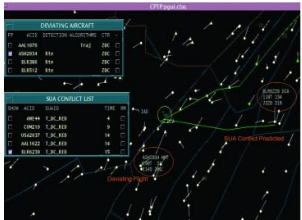
Figure 74: NASA's Rogue Evaluation and Coordination Tool provides real-time information about aircraft that deviate from their expected flight path, allowing air traffic controllers to identify collision risks or potential terrorist threats.
