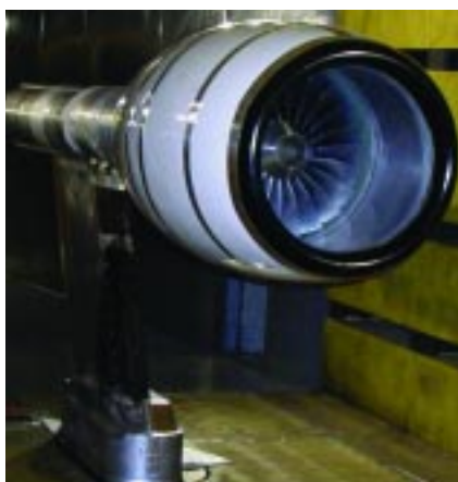
Figure 75: A fan designed to reduce aircraft noise is tested in a NASA laboratory.
