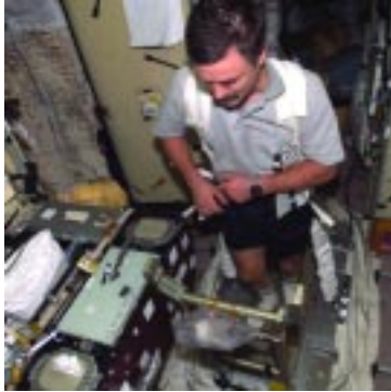
Figure 130: Expedition 8 Flight Engineer Alexander Y. Kaleri performs maintenance on the Treadmill Vibration Isolation System in the Zvezda Service Module on November 23, 2003.
