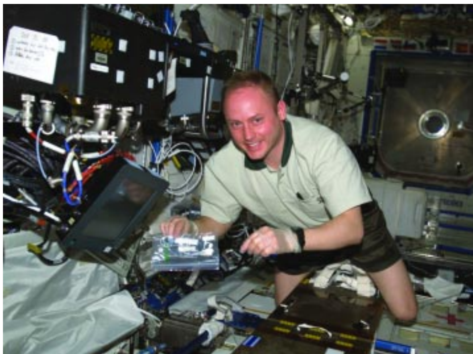
Figure 86: Expedition 9 Science Officer Mike Fincke works with equipment for the Binary Colloidal Alloy Test-3 experiment in the Station’s Destiny Laboratory on April 27, 2004. The experiment studied the long-term behavior of colloids—a system of fine particles suspended in a fluid like paint or milk—in a low gravity environment.
