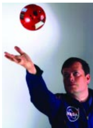
Figure 137: NASA's Personal Satellite Assistant is an autonomous, free-floating robot equipped with sensors to monitor environmental conditions inside a spacecraft or other enclosed environment.
