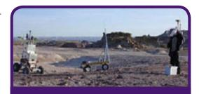
One of the Mobile Agents researchers, dressed in a spacesuit, looks at the computer network relay (center) and a robotic assistant called Boudreaux, which was being teleoperated by a handler. The spacesuits include a communication earpiece and microphone. (Photo: NASA/Mars Society)
