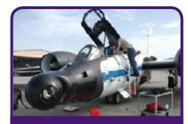
The WAVE project swiveling video recording system sits on the front of NASA's two WB-57 jets like a bulbous nose. The primary optic lens, a 4,150-millimeter reflector telescope, is visible on the right of the spherical turret. NASA partnered with Southern Research Institute, who design gimbal systems for the U.S. Army, to design a large, rotating gimbal to house the cameras that was stable and would remain focused on the speeding Shuttle. (Photo: NASA)
