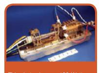
This photo shows a 100-Watt Ka-band traveling wave tube amplifier designed for NASA's 2009 Mars Telecommunication Orbiter mission. (Photo: NASA)
