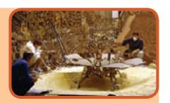
Rover engineers check how a test rover moves in material chosen to simulate the dune that bogged down *Opportunity* on April 26, 2005. They are working inside the In-Situ Instrument Laboratory at NASA's Jet Propulsion Laboratory. The team will use the information they gained from the tests and *Opportunity*'s observations of the dune to better direct the rover and to develop safer routes for future rover missions. (Photo: NASA)
