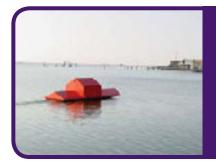
Looking like a floating doghouse, an OASIS aquabot maneuvers around open water during a test conducted in March 2005. Trailing behind the aquabot (not visible in the picture) was an operator in a chase boat who guided the aquabot with a remote control box. After the test, the team made changes to the propulsion motor/controller, which overheated during the test, to prepare the aquabot for the next phase of testing in the summer. (Photo: NASA)
