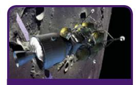
NASA's new exploration vehicle, shown in this artist's concept orbiting the Moon, will have solar panels to provide power. The capsule and the lunar lander will use liquid methane in their engines. NASA chose liquid methane as a fuel in anticipation of future Mars missions, where astronauts can convert Martian atmospheric resources into methane fuel. (Image: NASA/John Frassanito and Associates)
