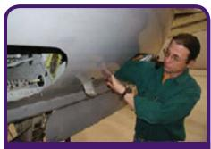
A technician installs a TAMDAR sensor in a Saab 340 commuter airliner at Mesaba Airlines. The Mesaba Airlines fleet will carry the sensors for a year as part of the Great Lakes Fleet Experiment, an operational test of the sensors' ability to provide timely weather forecasts. (Photo: D. Jackson/Mesaba Airlines)
