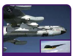
NASA's B-52B mothership carries the X-43A, attached to the nose of a Pegasus rocket booster, under its wing on November 16, 2004. The body of the small, slim X-43A (inset artist's concept) forms critical elements of the vehicle's design. The forebody acts as part of the intake for airflow and the aft section serves as the nozzle. (Photo: C. Thomas/NASA; drawing S. Lighthill)
