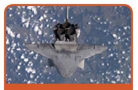
Discovery shows its belly in this photo taken by Station crew as the Shuttle backflips on July 28, 2005. The maneuver was added to Shuttle procedure so the Station crew could scan the heat shield for any damage caused during launch. The image was overexposed to bring out details of the individual black heat shield tiles, helping Station and ground crew search for anomalies. (Photo: NASA)
