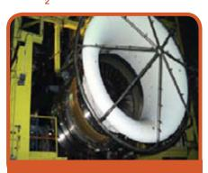
The engine shown above demonstrated a 50 percent reduction in NOx emissions during past tests conducted by NASA's program partner, Pratt & Whitney. (Photo: NASA)
