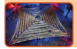
NASA engineers, visible near the bottom of the photo, look at a 20-meter solar sail and boom system after it is fully deployed during testing at NASA's Space Power Facility. Red and blue lights help illuminate the four triangular sail quadrants as they lie outstretched. The sail material is supported by a series of inflatable booms that become rigid in the space environment. The system extends via remote control from a central stowage container about the size of a suitcase. (Photo: NASA)
