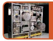
This photo shows the water recovery system for the International Space Station's Environmental Control and Life Support System in 2000. NASA engineers are developing smaller, lighter, and more efficient technologies to reduce the mass of all life support systems for the Station and future space exploration spacecraft and surface habitats. (Photo: NASA)
