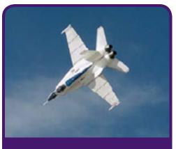
NASA's F/A-18A maneuvers through a test point for the Active Aeroelastic Wing project on December 15, 2004. The stock aircraft was modified with a thinner, more flexible wing skin and structure, new flight control computer software, and a number of sensors that track the wings' flexibility and strain. (Photo: NASA/C. Thomas)
