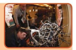
A NASA research team installs a sphere containing 50 sensitive microphones in the cabin of a 757 jet to isolate the sources of noise that are irritating to aircraft crew and passengers. This testing helps engineers develop planes that are quieter and more comfortable. (Photo:
