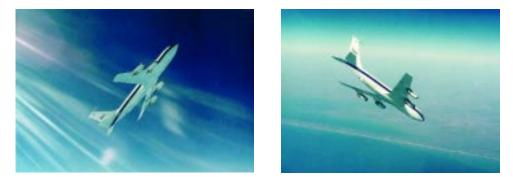
Figure 42: A typical flight mission on a KC-135 lasts about two to three hours. During each steep dive, the passengers experience 20 to 25 seconds of reduced gravity.
