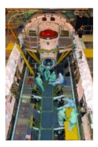
Figure 2: Crews install an orbiter Boom Sensor System in *Discovery's* bay on June 10, 2004. The OBSS, a new return to flight safety measure, includes cameras and laser systems attached to a long crane-like boom that can inspect the Shuttle's thermal Protection System during flight.
