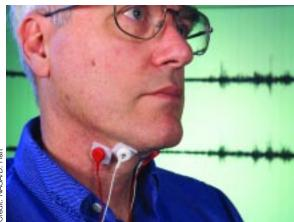
Figure 58: NASA scientist Chuck Jorgensen models the sensors, worn under the chin and on either side of the "Adam's apple," used to gather nerve signals that control speech.
