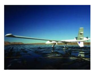
Figure 57: The remotely-piloted Altair uncrewed aerial vehicle was developed for NASA by General Atomics Aeronautical Systems, Inc. as a long-endurance, high-altitude platform for development of UAV technologies and environmental science missions.
