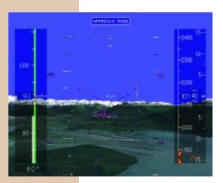
Figure 20: Simulations and flight studies show that the Synthetic Vision System increases pilot situational awareness and reduces errors and workload.
