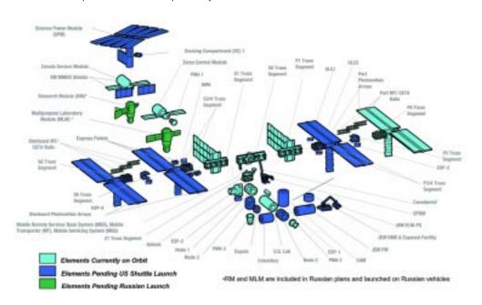
Figure 23: The ISS technical station configuration endorsed at the July 2004 meeting.
