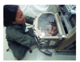
Figure 41: NASA Explorer School educator Alissa Kuseske uses a small glovebox to perform her students' spinning tops experiment onboard the KC-135. The glovebox kept the tops from floating around the cabin during the jet's roller coaster-like dives.
