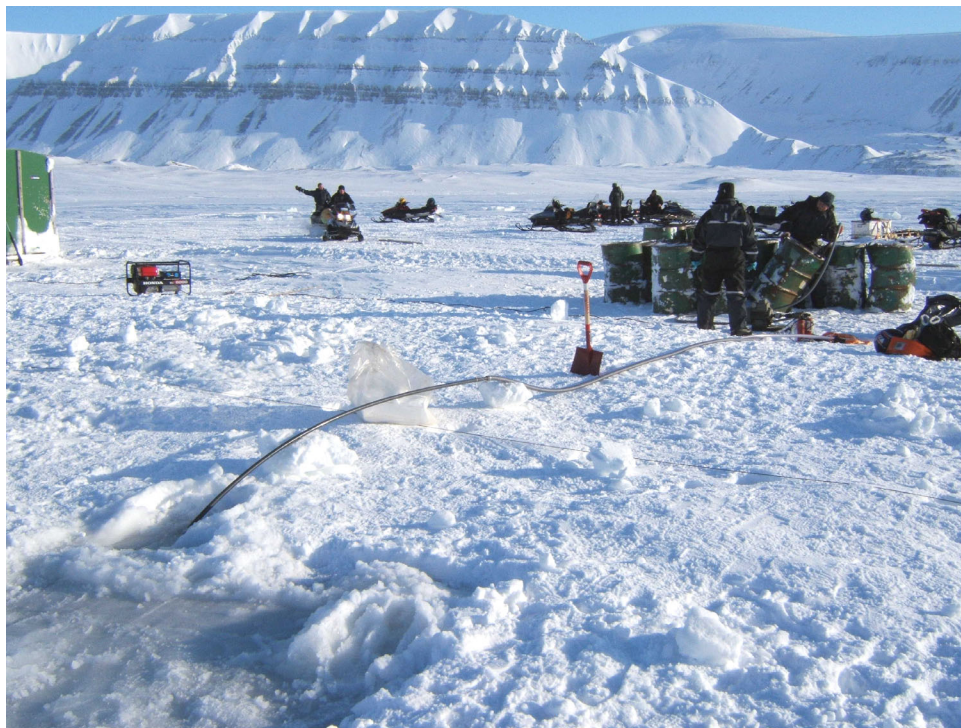
Pumping oil from drums through flexible pipe inserted 1 m inside skirt through a sloped hole drilled 2 m outside
