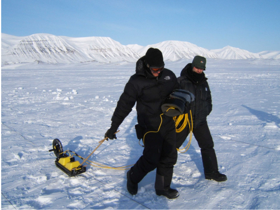
Radar surface traverse along a marked survey line
