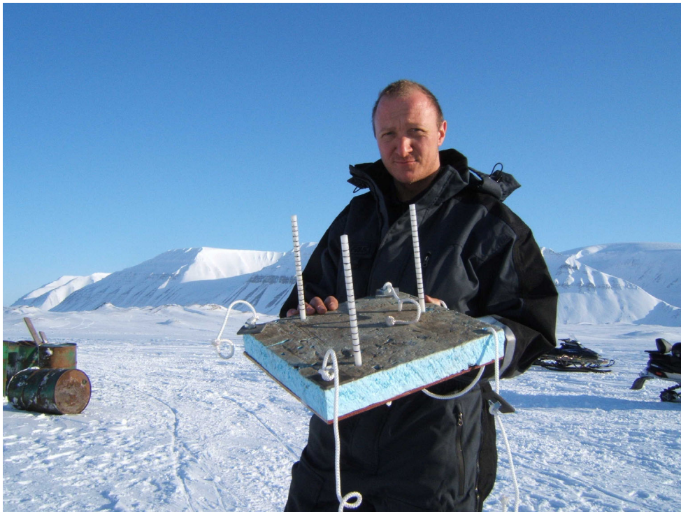
SINTEF prototype under-ice oil thickness sampler
