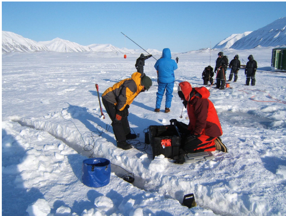
Testing the acoustics system by moving the transducer along a trench straddling clean and oiled ice. Water was used to wet the ice to improve coupling.
