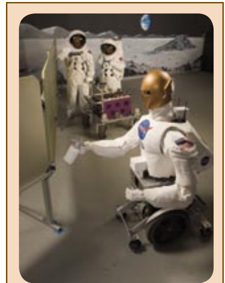
In November 2005, Johnson Space Center's Robonaut (foreground) performs a mock weld while Ames Research Center's K10 robot assists two spacesuited crewmembers inspecting a previously welded seam. This activity tested human-robot interactions and the two robots' ability to work together autonomously for assembly and maintenance, important capabilities for future lunar exploration. (NASA)
