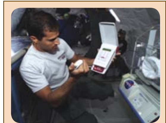
NASA is developing Advanced Environmental Monitoring and Control systems for flight on the ISS (and ultimately Orion) to detect harmful contaminants in the atmosphere and alert the crew. In this photo, project scientist Jake Maule uses the Lab-on-a-Chip Application Development (LOCAD)-Portable Test System, a hand-held device for rapid detection of potentially harmful biological and chemical substances, aboard NASA's KC-135 microgravity research aircraft. (NASA)
