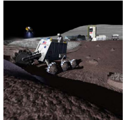
To minimize the consumables that must be launched from Earth to sustain a lunar outpost, in-situ resources will be used to produce oxygen, water, and propellants. This picture shows an artists conception of a lunar rover excavating regolith for chemical processing in a nearby in-situ resource utilization facility.
