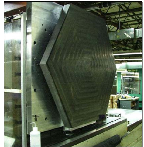
18 hexagonal mirror segments are fabricated in batches of approximately six at a time. The total effort takes roughly 4.5 years. The segments have 3 prescriptions of six mirrors each and assembly line techniques can be used to make the mirrors in parallel. The 18 segments are aligned in space using special algorithms being developed and demonstrated on testbeds on the ground.
