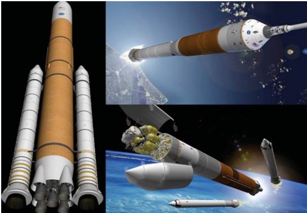
An artist's conception of the Constellation Systems. Far left: The Heavy Lift Launch Vehicle (HLLV) to launch Lunar bound systems, Top : CEV atop the CLV, Bottom: Earth Departure Stage launched on HLLV.
