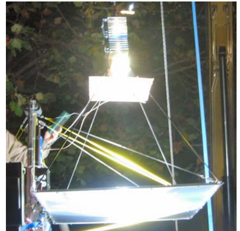
Beam Power Competition Entry - Robotic climber is using wireless power at NASA's first Centennial Challenges prize competition.
