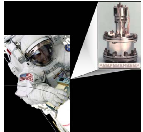
TGA (trace gas analyzer) - used by astronauts in Shuttle Mission 5A and beyond to detect ammonia and air leaks outside the International Space Station. Contains the Quadrupole Mass Spectrometer
