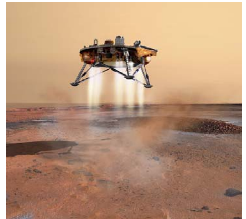
Phoenix landing thrusters provide a gentle touchdown on the Martian surface. (artist's representation)
