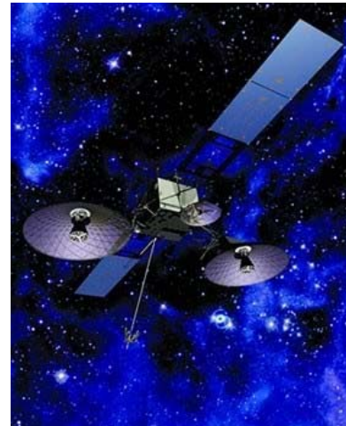
The Tracking and Data Relay Satellite (TDRS) shown above represents a constellation of 8 operational satellites providing uplink and downlink capability for NASA and non-NASA missions.
