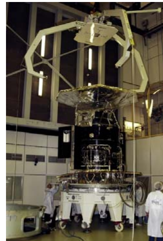
Herschel Payload Module leaving the Large Space Simulator (LSS) after the Thermal Blanket / Thermal Vacuum (TB/TV) test.
