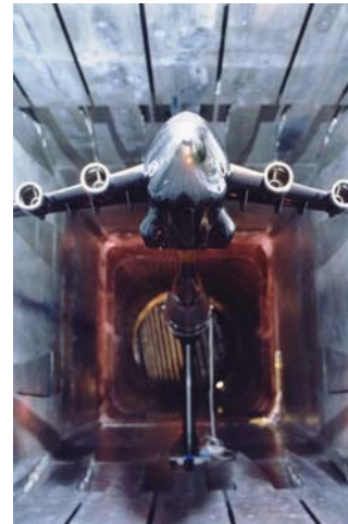
This high-wing transport aircraft model was used in the National Transonic Facility (NTF) to evaluate aerodynamic performance at flight conditions. NASA has many Aeronautics test facilities, including wind tunnels, propulsion test cells, and simulators, that are considered national assets.
