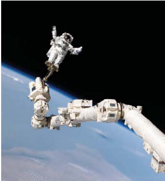
Astronaut Stephen K. Robinson, STS-114 mission specialist, anchored to a foot restraint on the International Space Station's Canadarm2, participates in the mission's third session of extravehicular activity. The blackness of space and Earth's horizon form the backdrop for this image.
