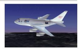
Artist's concept of SOFIA in flight with cavity door open and telescope visible.
