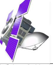
CloudSat has a nadir pointing radar optimized to penetrate clouds and reveal their interior water and aerosol content.
