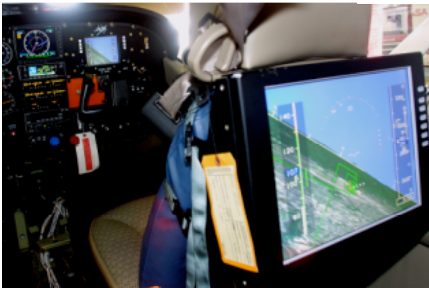
New cockpit displays can paint a picture of the outside world so pilots can land safely even in bad weather.
