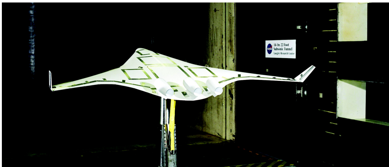
A scale model of an early blended wing body design was tested in one of the NASA Langley wind tunnels.
