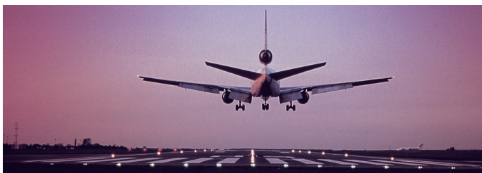
Landing gear, slats and flaps are the primary source of airframe noise
