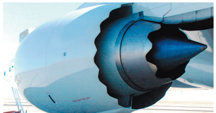
Scalloped edges around engine nozzle mix the jet exhaust and reduce noise.
