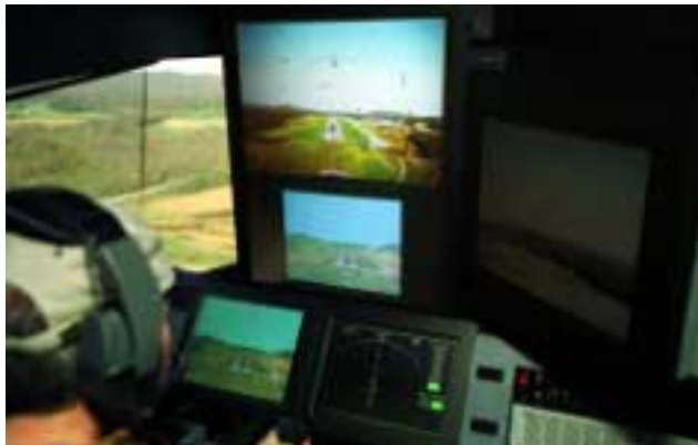
During a flight test, a NASA research pilot compared a terrain database (bottom) to the real world.
