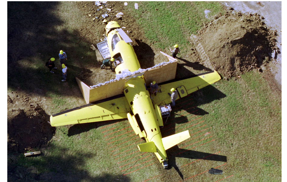
NASA engineers dropped a Lear Fan composite aircraft 150 feet to test whether design changes can help pilots and passengers better survive an accident.
