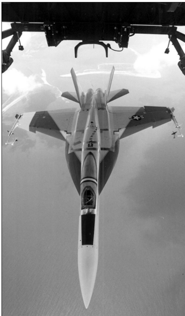
Remotely piloted drop model tests probe the limits of the flight envelope.
