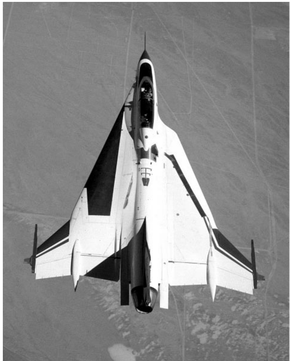
F-16XL with supersonic laminar flow control experiment (black area on left wing, front) or "glove."
