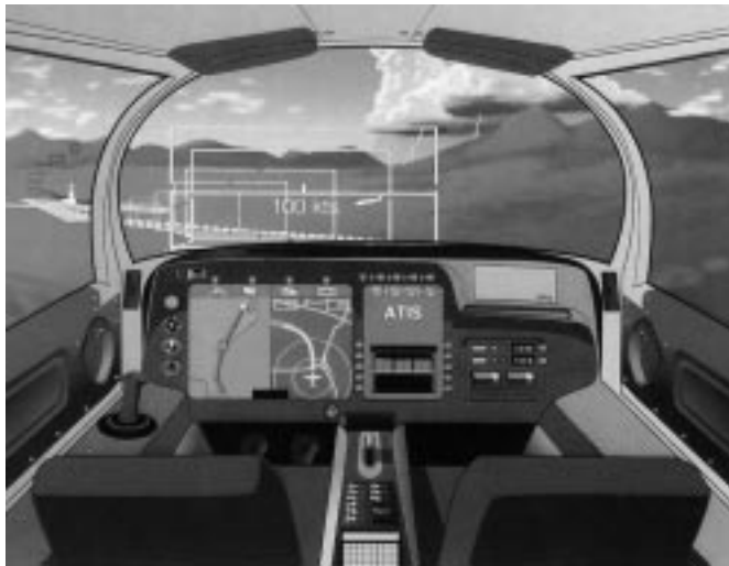
Next-generation general aviation cockpit with single lever power control. The system will utilize a computer that provides up-to-date weather reports, the latest in airways and facilities information, and map displays that point out restricted areas, terrain hazards, airports, and airspace conditions.
