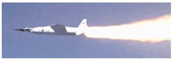
A modified Pegasus booster rocket ignites moments after release from the B-52B, beginning the acceleration of the X-43A over the Pacific Ocean in March of 2004. The X-43A vehicle is mounted on the nose of the rocket.
