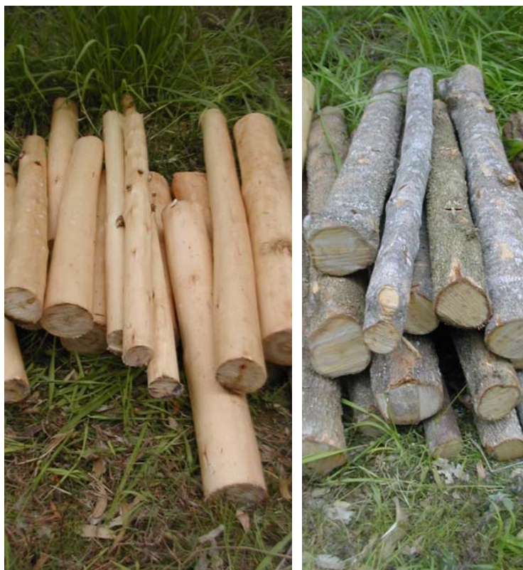
Figure 1. Bolts of debarked E. grandis that were processed for use in gasifier tests are shown at left. E. grandis with bark intact is shown at right.
