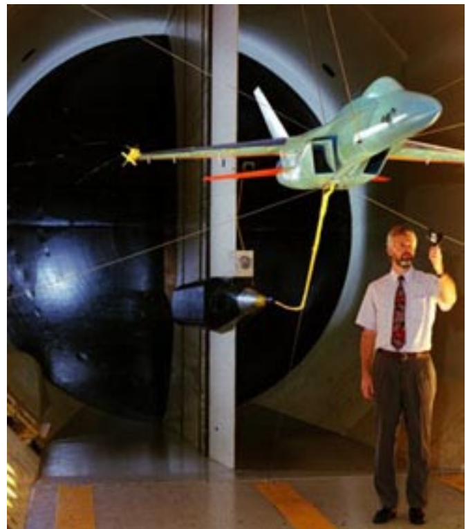
F/A-18 E/F flutter clearance model in the NASA Langley Transonic Dynamics Tunnel.
