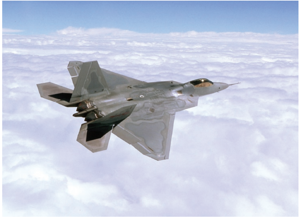
The Air Force F-22 fighter uses thrust vectoring technology that evolved from Langley's pioneering research.
