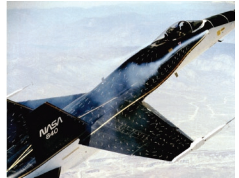
Flow visualization studies using tufts and smoke identify flow phenomena on the NASA F-18 High Alpha Research Vehicle at high angles of attack.
