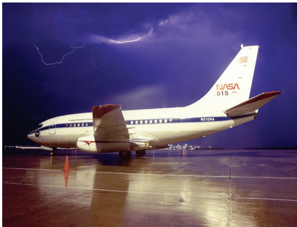
Langley's 737 research aircraft provided validation data and demonstrations of the effectiveness of airborne detection concepts by flying windshear missions.
