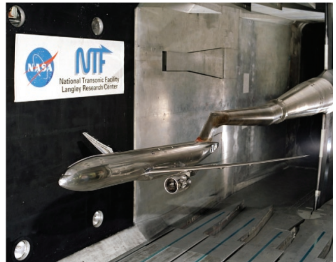
Model of the Boeing 777 transport undergoing tests in the National Transonic Facility at Langley .
