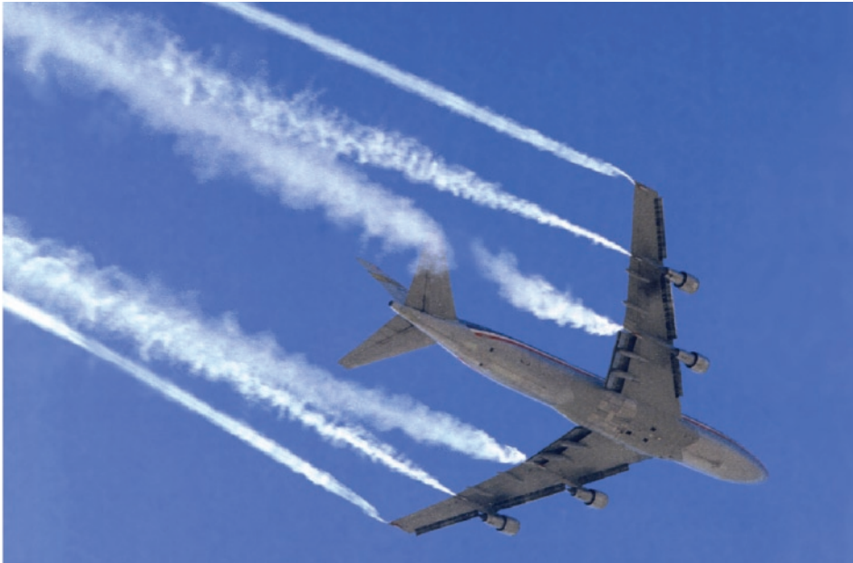
Smoke injected into the trailing vortices of a Boeing 747 transport during NASA flight tests of wake vortex alleviation concept.
