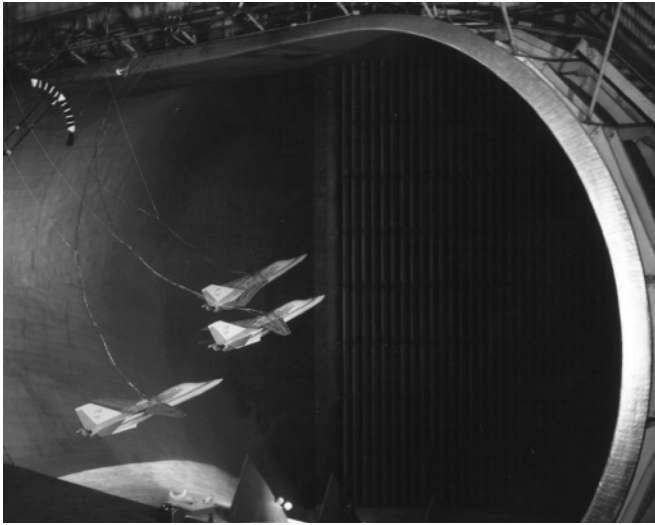
Time sequence photographs of an F-111 model being assessed with various wing sweep angles during free-flight tests in the Langley Full-Scale Tunnel.
