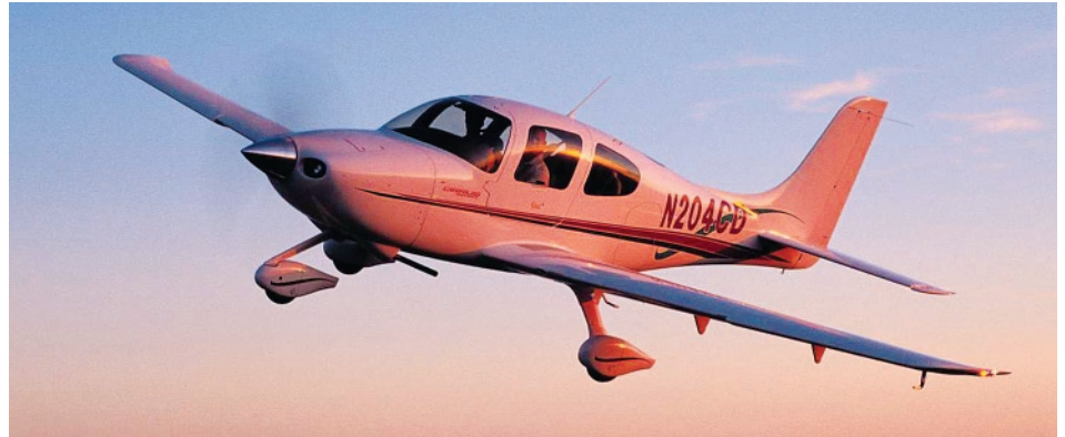
A composite fuselage structure is used on the Cirrus SR-20 general aviation aircraft.
