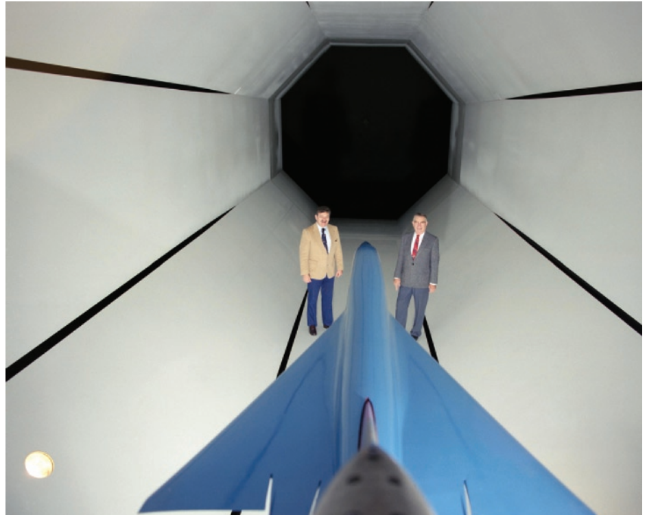
Slotted-throat test section of the Langley 16-Foot Transonic Tunnel.
