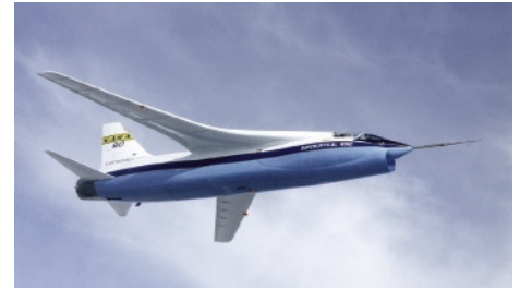
NASA's F-8 supercritical wing research airplane in flight at the NASA Dryden Flight Research Center.
