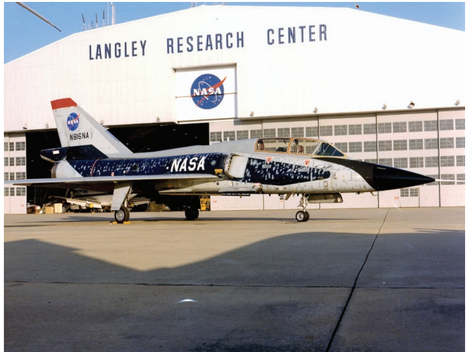
F-106 research aircraft used by Langley for lightning characterization research. Gray marks on airplane are paint marks denoting lightning strike points.
