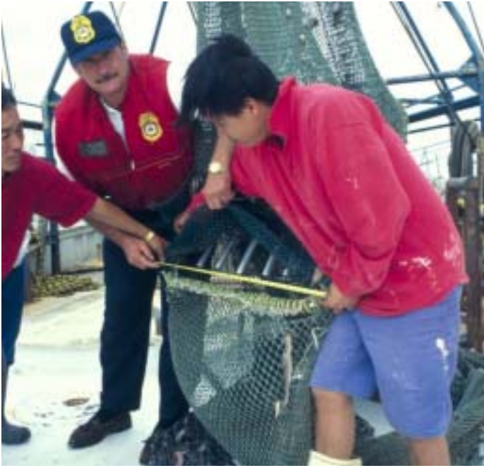
An officer measures the opening of a Turtle Excluder Device to ensure that it meets federal guidelines. Dockside inspections like this help ensure compliance with a variety of fishery regulations.
