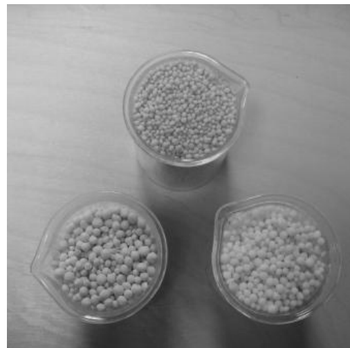
Figure 1. Urea + Agrotain (top), ammonium nitrate (bottom left), and Super U (bottom right).
