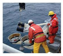
Bongo nets are one of the methods used to collect fishery data
