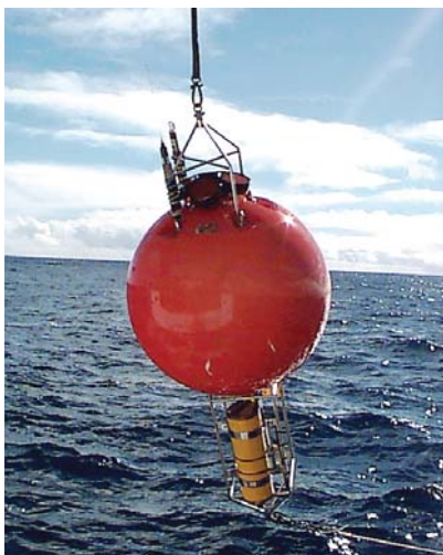
Acoustic Doppler current profiler is deployed to measure ocean currents
