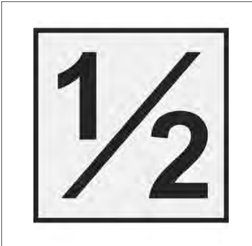
FIG 7-5-1 Typical Runway Half-way Sign
