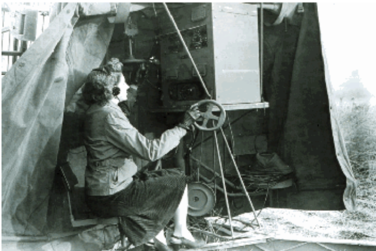
SCR-658 radio direction finder used to track radiosonde balloons. Woman observer indicates WWII or just after war time frame. World War II expanded the opportunities for women in the Weather Bureau. Photo Date: 1945-1946
