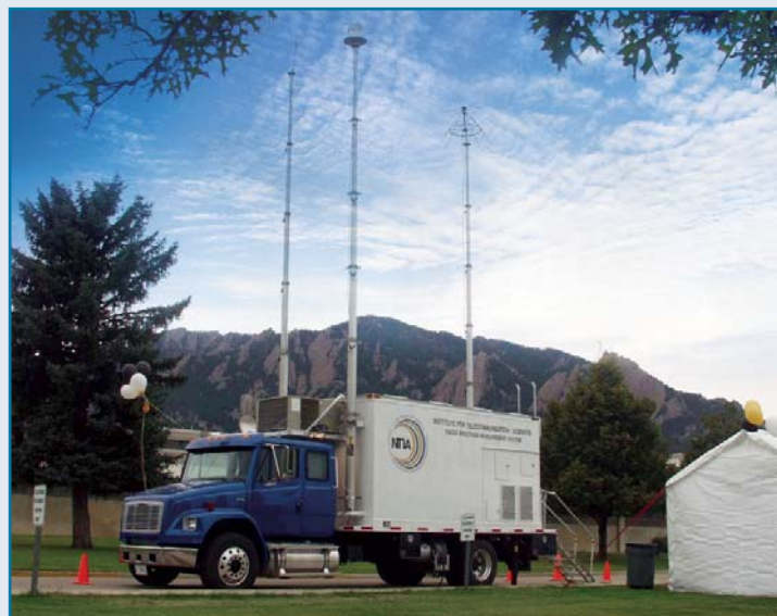
The NTIA Institute for Telecommunication Sciences' 4th generation Radio Spectrum Measurement System (RSMS) is equipped with state-of-the-art instrumentation, measurement methods, and analysis capabilities to support federal spectrum management, usage assessments, interference resolution, propagation research support and other federal agency needs.
