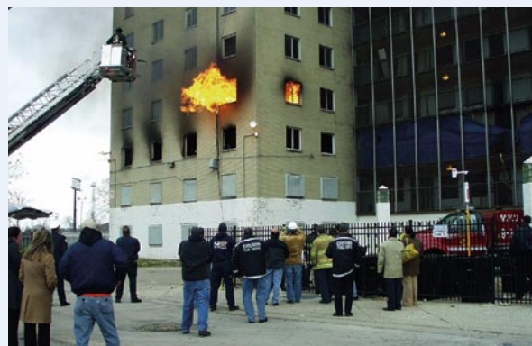
Members of a NIST research team watch flames erupt from an abandoned Chicago apartment building during a November 10, 2006 test of PPV in high-rise fires.
