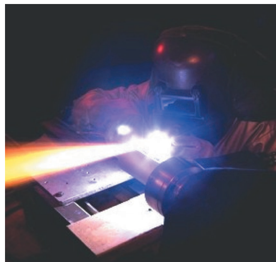
The PS304 coating is plasma sprayed on the bearing shaft.
