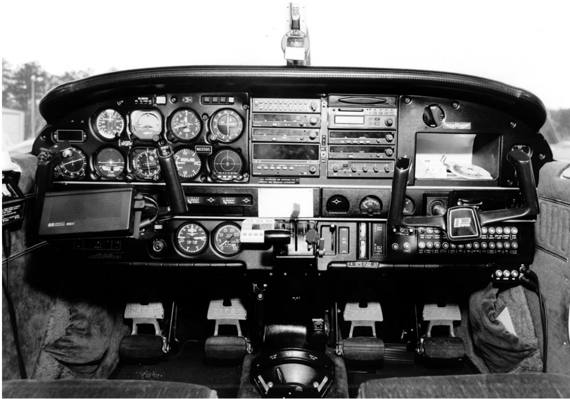
In current general aviation aircraft, several levers are used for engine power control (as seen on center console unit).
