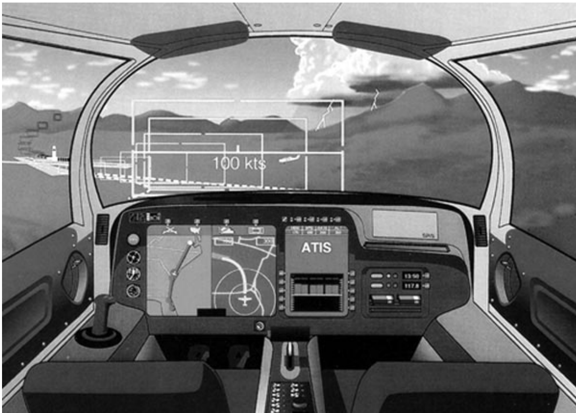
The use of a single lever for power control in retrofitted and future aircraft reduces the number of flight-related displays in the instrument panel, thus increasing pilot awareness.
