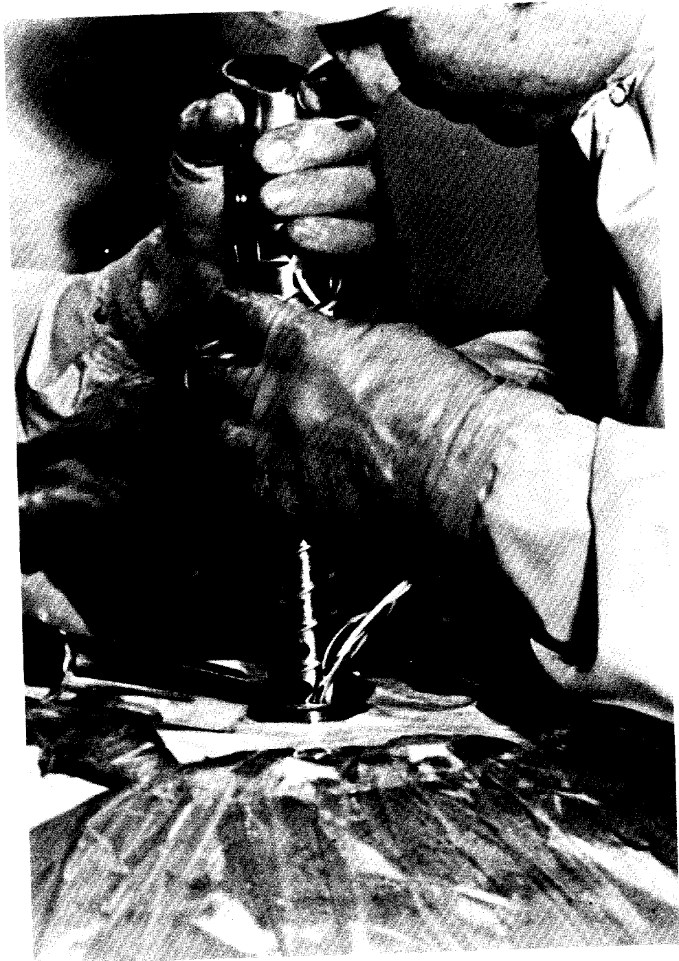
Figure C4-32.- Feeding wires into tank beside heater probe.
