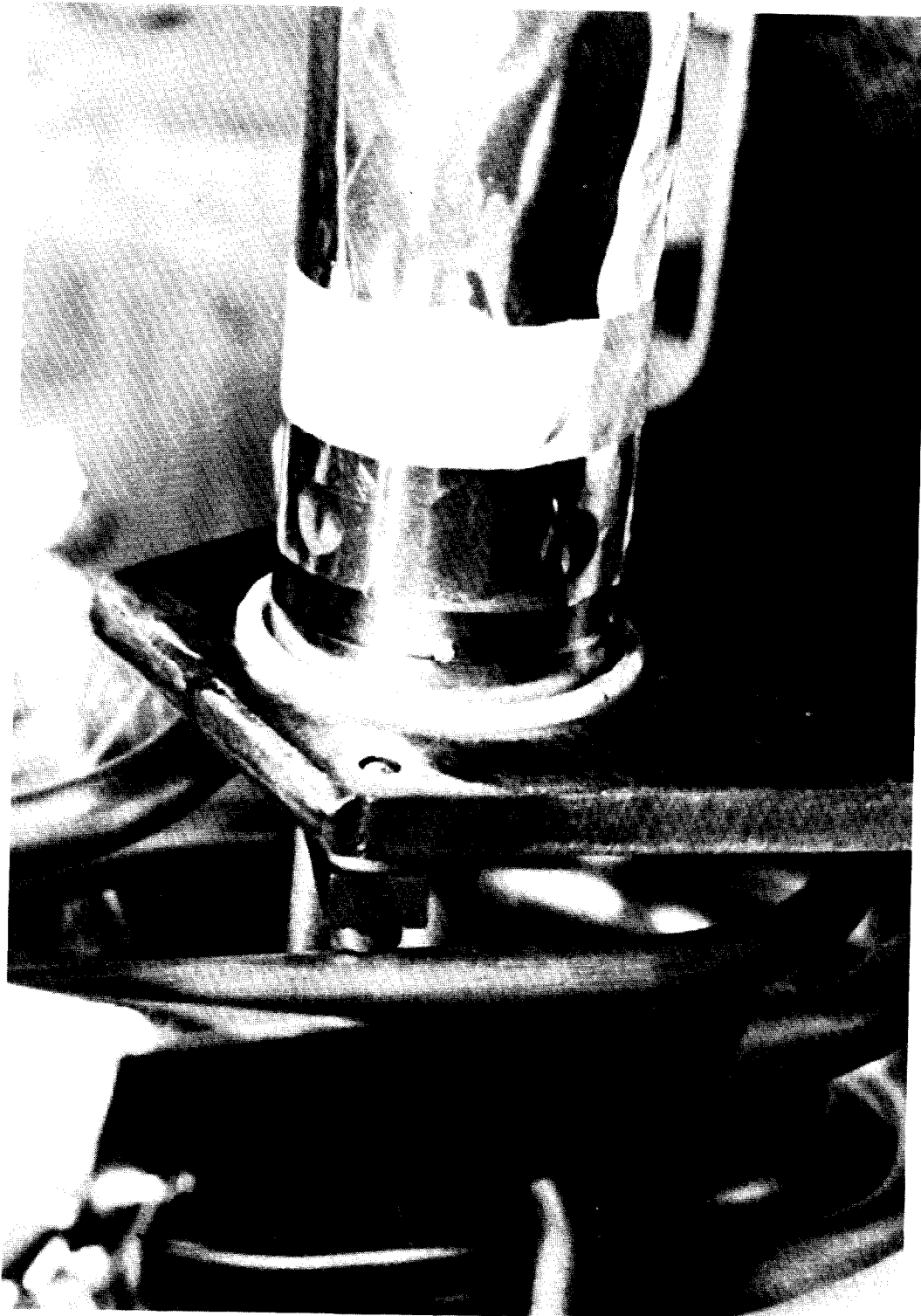
Figure C4-29.- The completed quantity probe to coil assembly welds.
