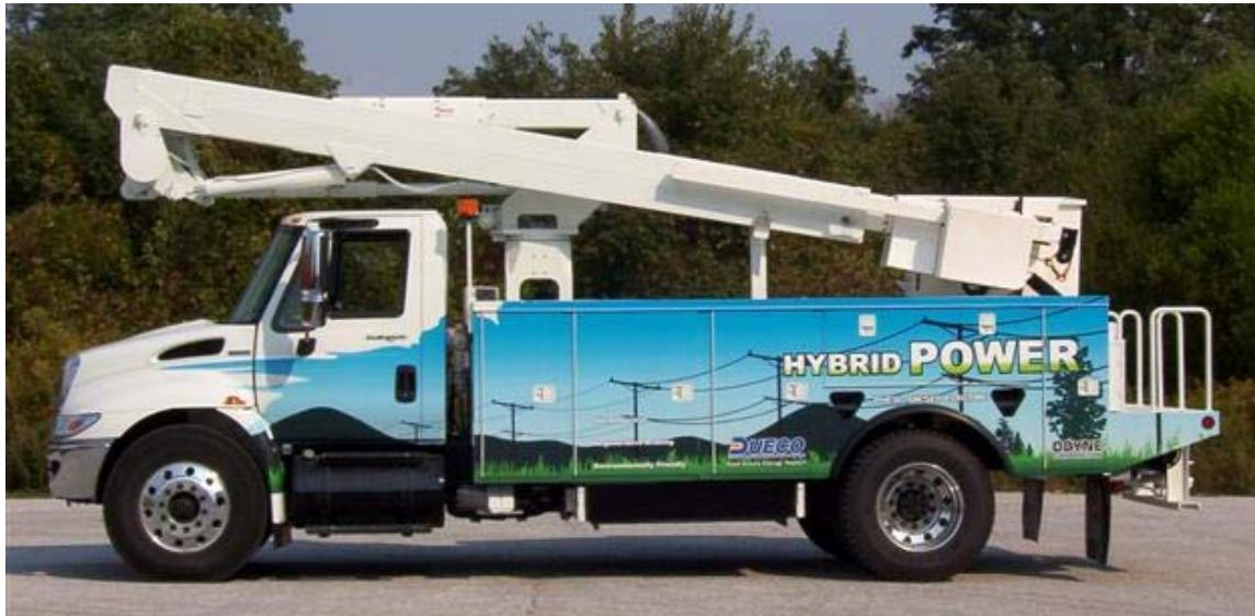
A plug-in hybrid electric medium duty bucket truck is shown above. This type of truck is typically used by utilities for maintenance and installation of power lines. The truck has many of the benefits listed previously. Specifically this vehicle has the following features:
