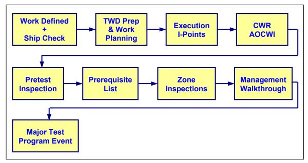
Figure 3.9 High-Level View of Nuclear Maintenance Assurance Process
