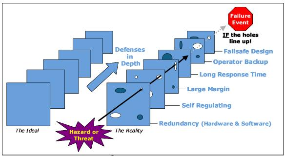
Figure 3.5 Multiple Barriers to Failure<sup>2</sup>
