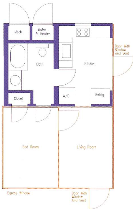
Figure 1. REFS Temporary 2-Room Shelter w/Bath and Kitchen Modules
