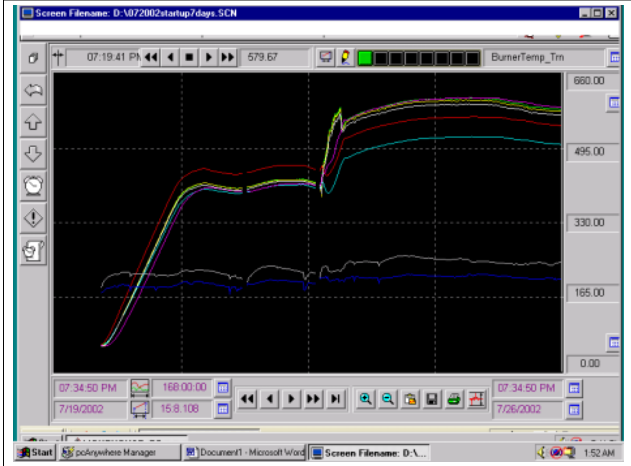
Figure 7. Fuel cell temperatures during startup.
