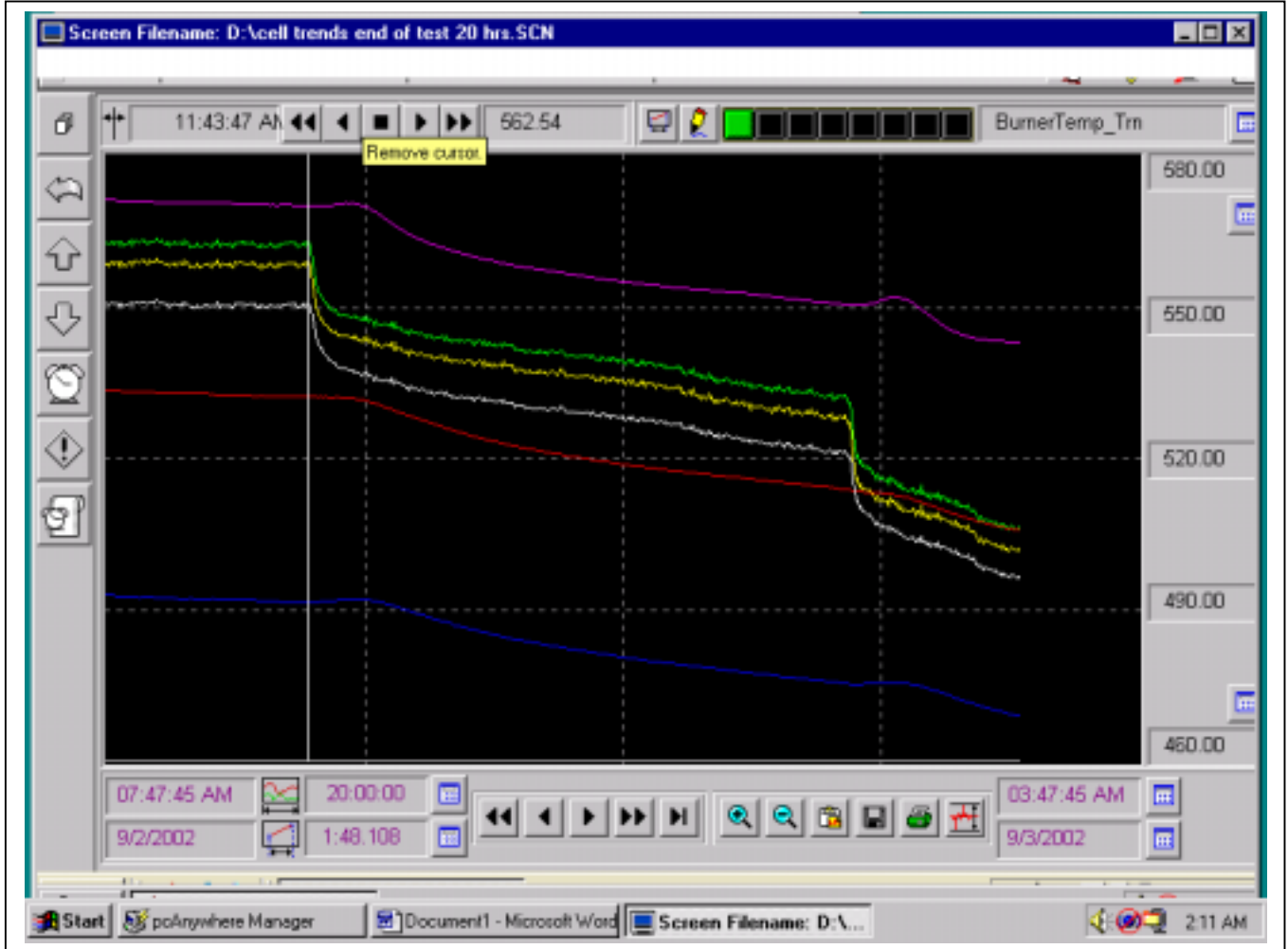
Figure 11. Low temperature shutdown plot.
