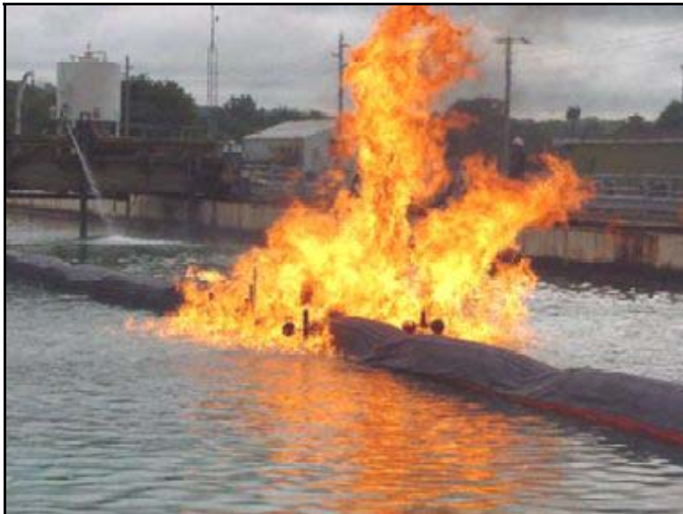
Figure C-14. Water-Cooled Fire Boom During Burn.
