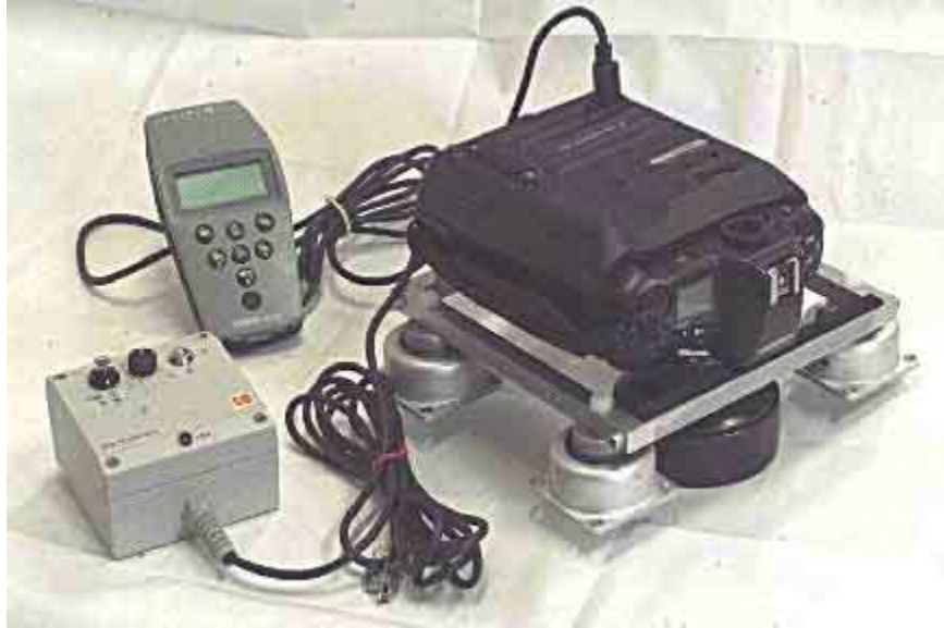
Camera mount and GPS connection used by Infoterra of Farnborough, UK.
