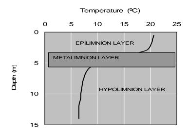
Figure 2. Thermal stratification schematic drawing.
