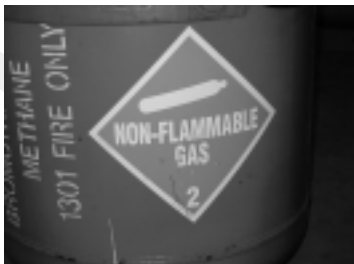
This "Non-Flammable Gas" label is one of the requirements when shipping halon. U.S. Department of Transportation (DOT) regulations for shipment of hazardous materials apply to halon shipments. Photo courtesy of U.S. DOD/DLA ODS Reserve.
