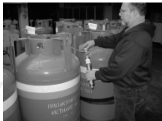
Technician taking a sample of Halon 1301. Recycled halon should be tested by an independent laboratory to ensure product conformance to specifications. Photo courtesy of U.S. DOD/DLA ODS Reserve.
