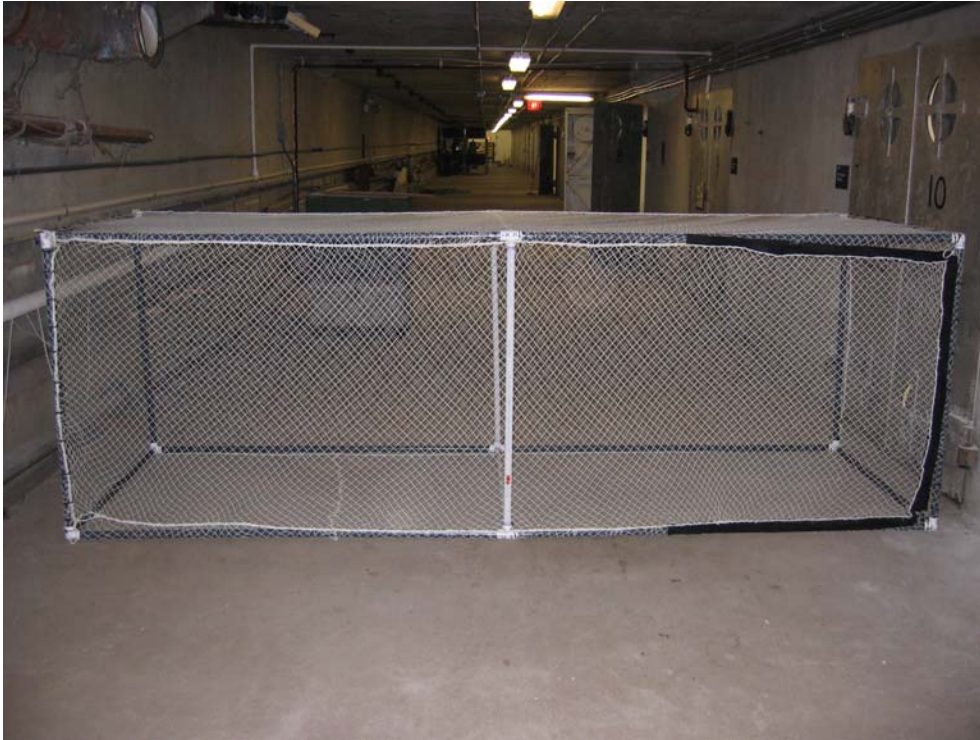
Fig. 2. Photograph (unmodified but reduced to page scale) of an experimental pen just after construction. Measurements are 3.7 x 1.2 x 1.2 m.
