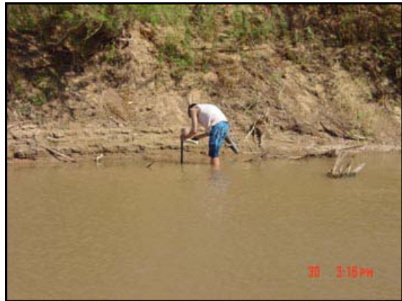
Setting up the thermograph to take hourly river temperature readings
