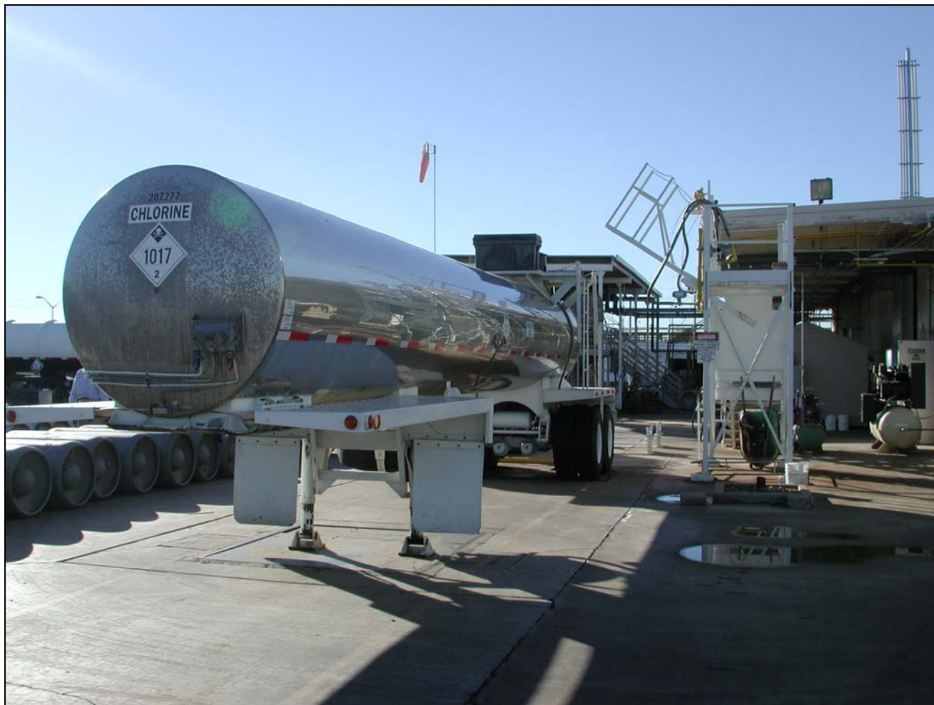
Figure 4. Chlorine bulk road trailer
