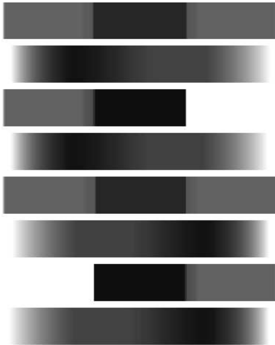
Figure 4.6: T-joint simulated radiographs at 45° increments.
