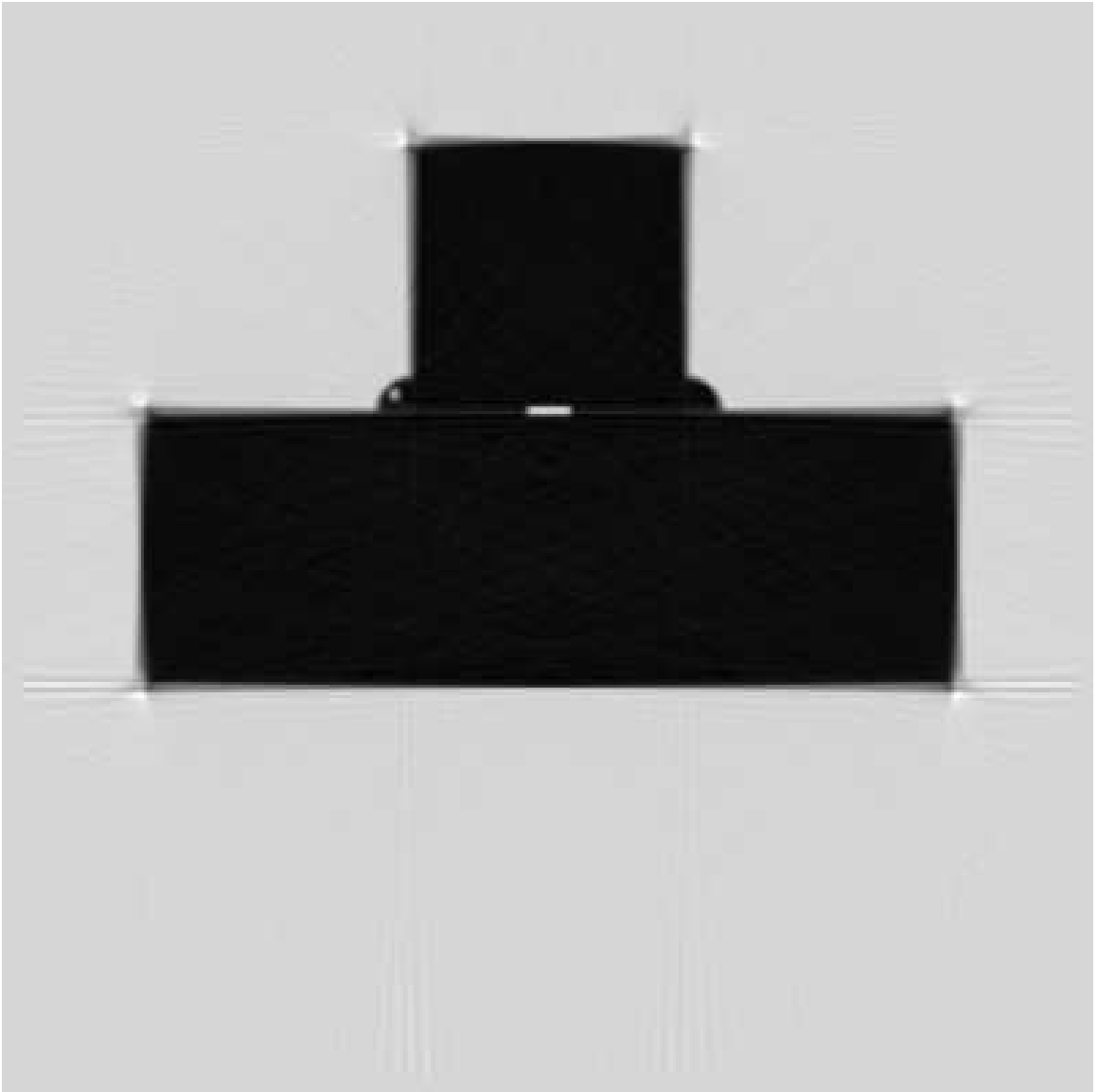
Figure 4.7: T-joint reconstruction from simulated data, 315 directions.
