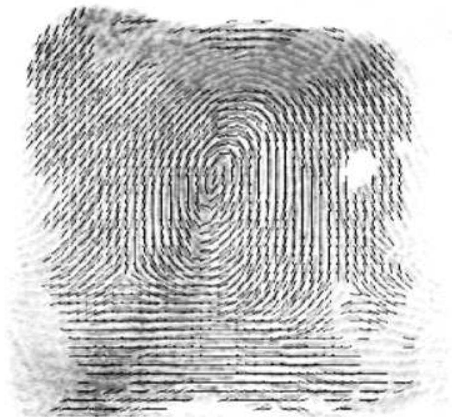
Figure 7.14: Tangent directions calculated on a 10 row by 8 column grid using a 19 row by 15 column tangent averaging window. Unmarked regions indicate either the contrast or the consistency is poor.
