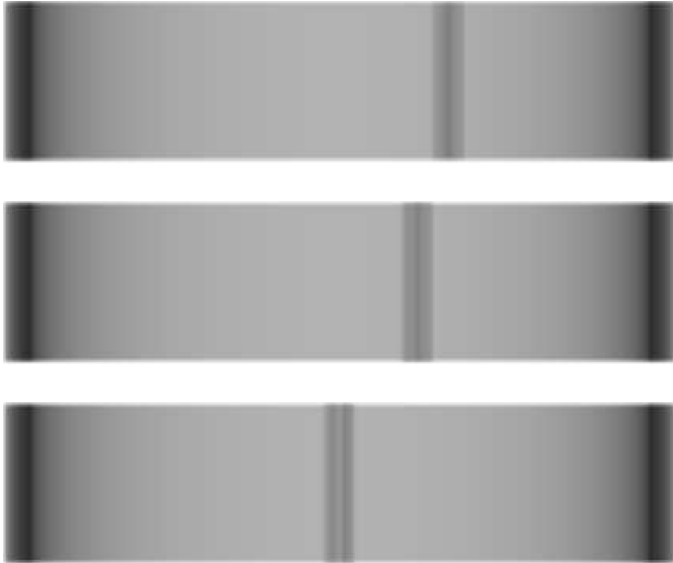
Figure 2.10: Simulated radiographs of the experimental sample: 0^\circ , 45^\circ , 90^\circ (top to bottom).
