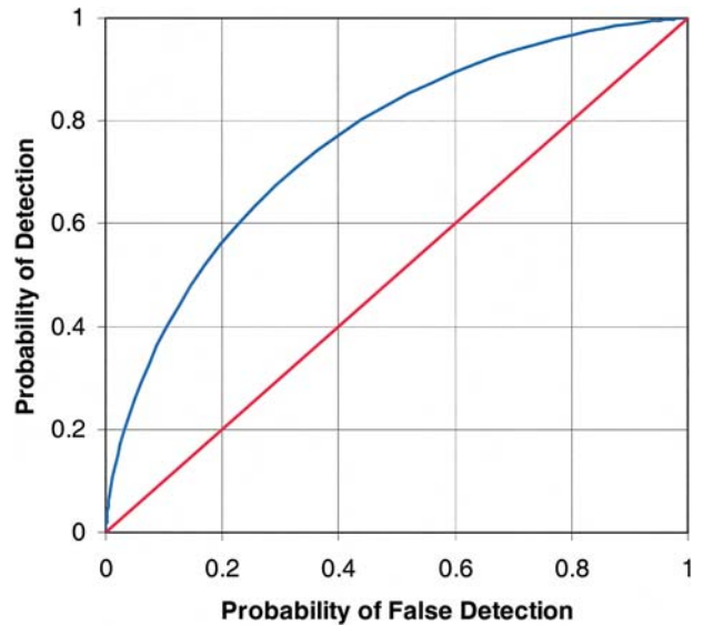
FIG. 2. The ROC curve associated with the model distribution shown in Fig. 1. The curved blue line is the plot of POD vs POFD for each decision threshold, and the 45° angle red line represents no skill.
