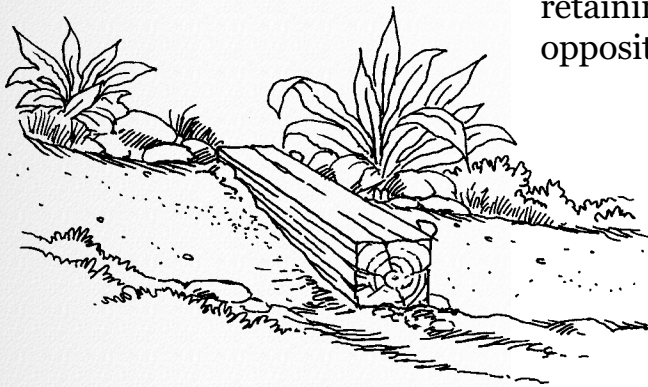
Figure 15-18. Non-flexible waterbars, such as a piece of wood or a log, are barriers for people with mobility impairments.
