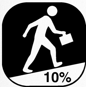
Figure 6-4. This type of sign is provided in some trail environments. Pedestrians could benefit from objective sidewalk information such as this sign that indicates an upcoming steep grade.
