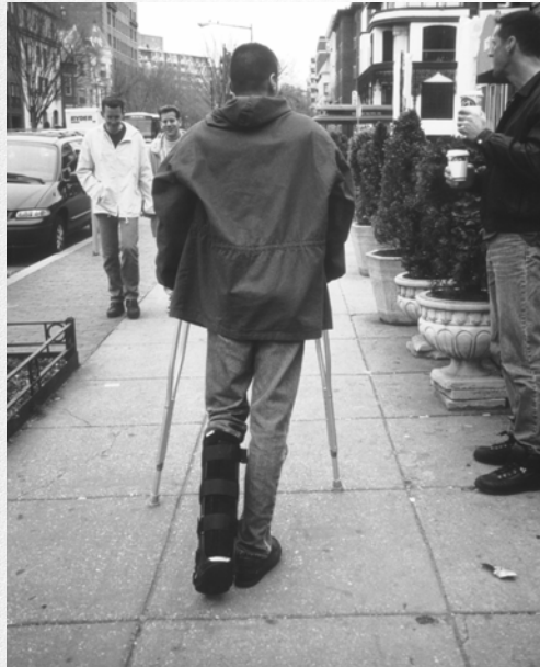
Figure 4-5. A minimum width of 1.525 m (60 in) is recommended for the pedestrian zone. This width should be completely free of obstacles and protruding objects.
