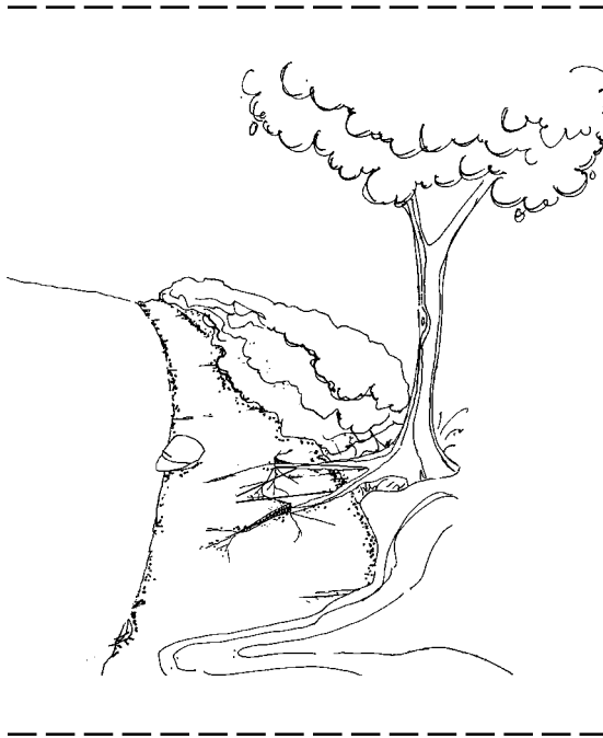
Figure 5-5: Tree roots that break up the surface of the trail should be removed because they can cause users to trip.
