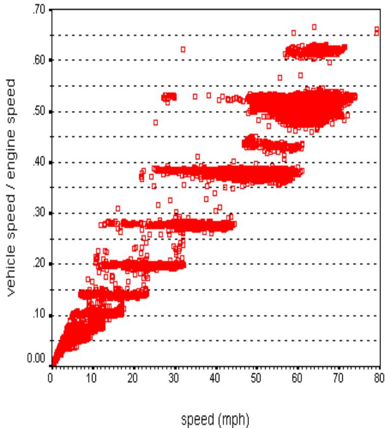
CE-CERT truck 1 vehicle speed to engine speed ratios plotted against vehicles speed to determine average speeds for a given gear
