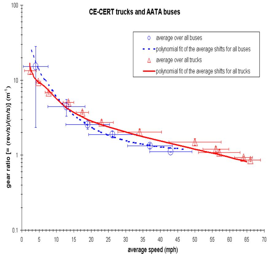
Final engine speed - vehicle speed relationships for buses (red) and the heavy duty trucks (blue). The error bars are standard deviations determined from the distributions depicted in vehicle speed - engine speed ratio graph
