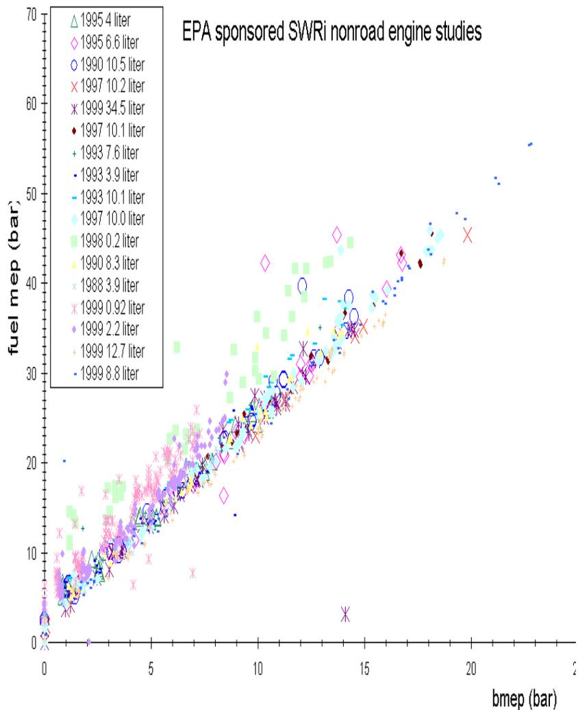
nonroad dynamometer based measurements of fuel consumption and brake mean effective pressure
