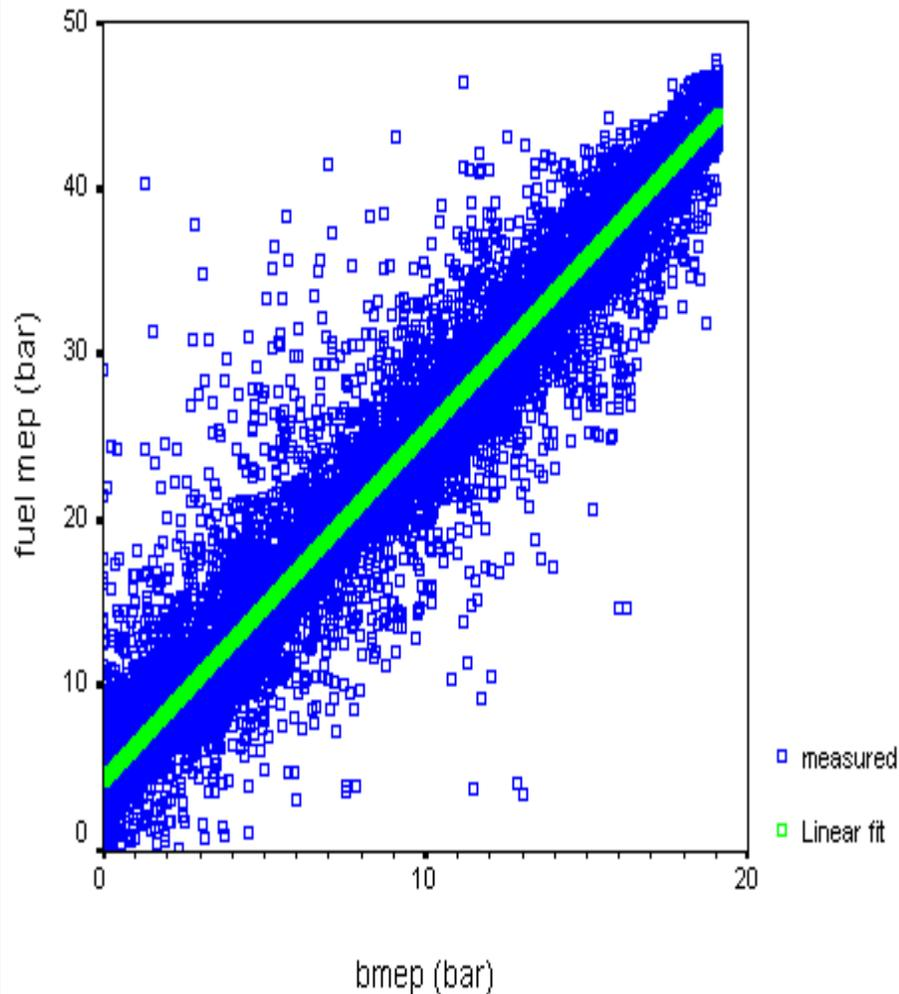
CE-CERT truck 1 on road based measurements of fuel consumption and brake mean effective pressure using engine maps and % load
