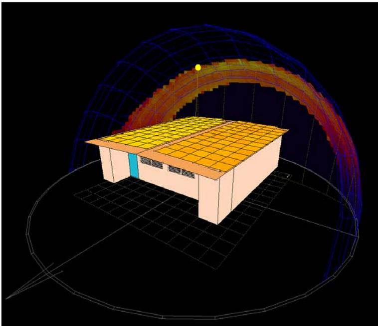
Fig. 30 – Solar Stress Simulation on P-26 using Ecotect.
