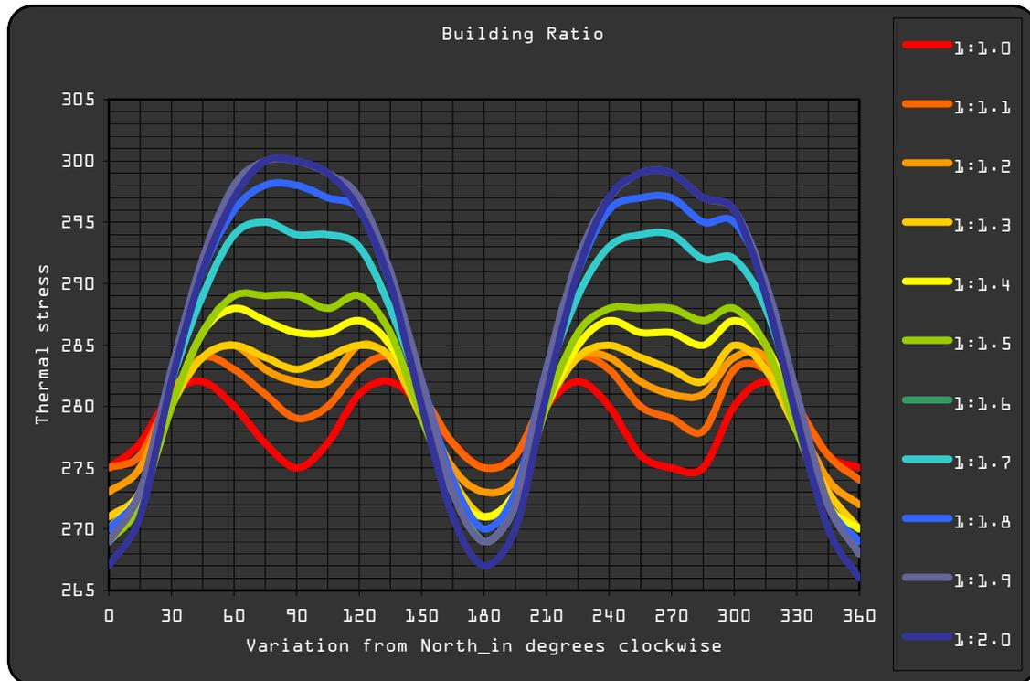
Fig. 37 – Solar Stress versus Building Proportion Ratios.
