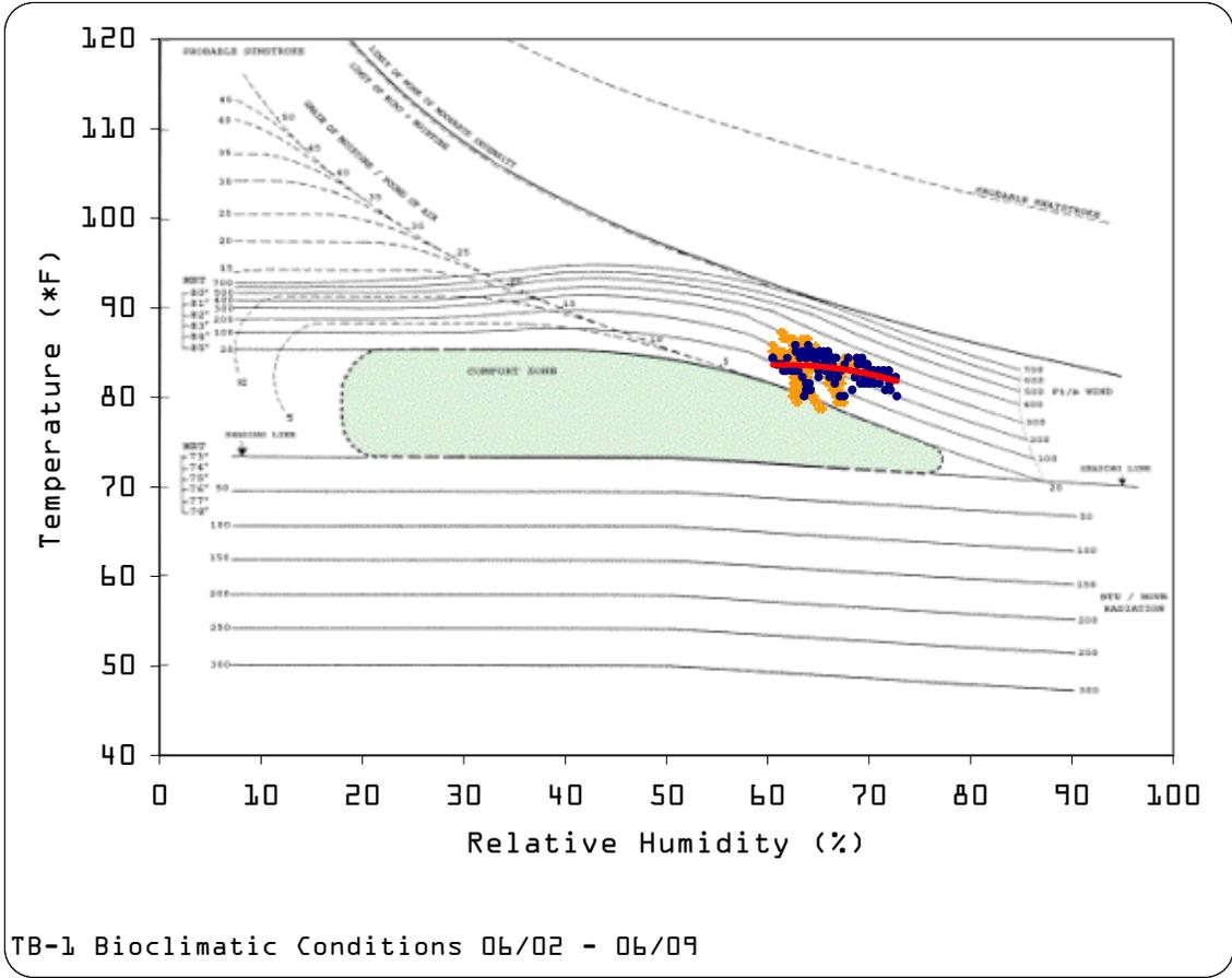
Fig. 27 - Bioclimatic Chart of TB-1 from 06/02/03 to 06/09/03.
