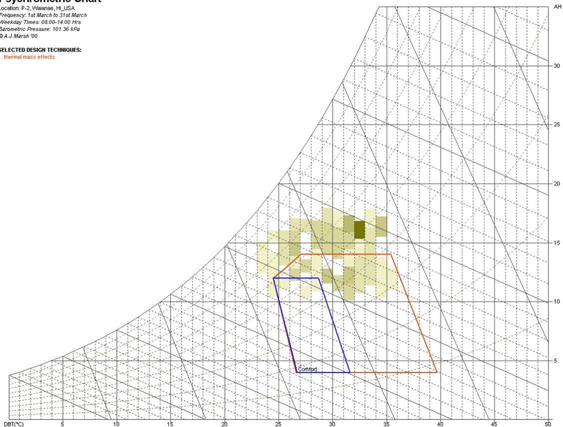
Fig. 33 – Increased Comfort Zone in P-2 through Thermal Mass Effect.
