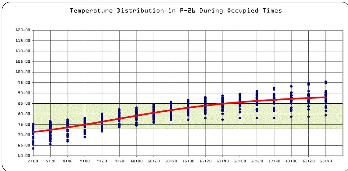
Fig. 11 – Temperature Distribution [occupied times] of P-26 from 10/25/02 to 12/20/02.
