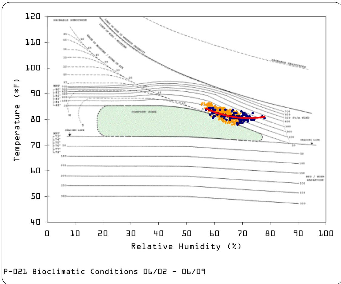
Fig. 24 - Bioclimatic Chart of P-021 from 06/02/03 to 06/09/03.
