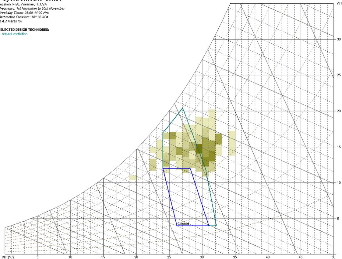
Fig. 34 – Increased Comfort Zone in P-26 through Natural Ventilation.
