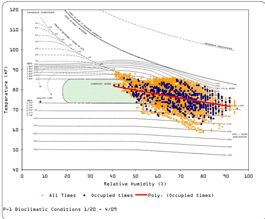
Fig. 16 - Bioclimatic Chart of P-1 from 01/20/03 to 04/09/03.
