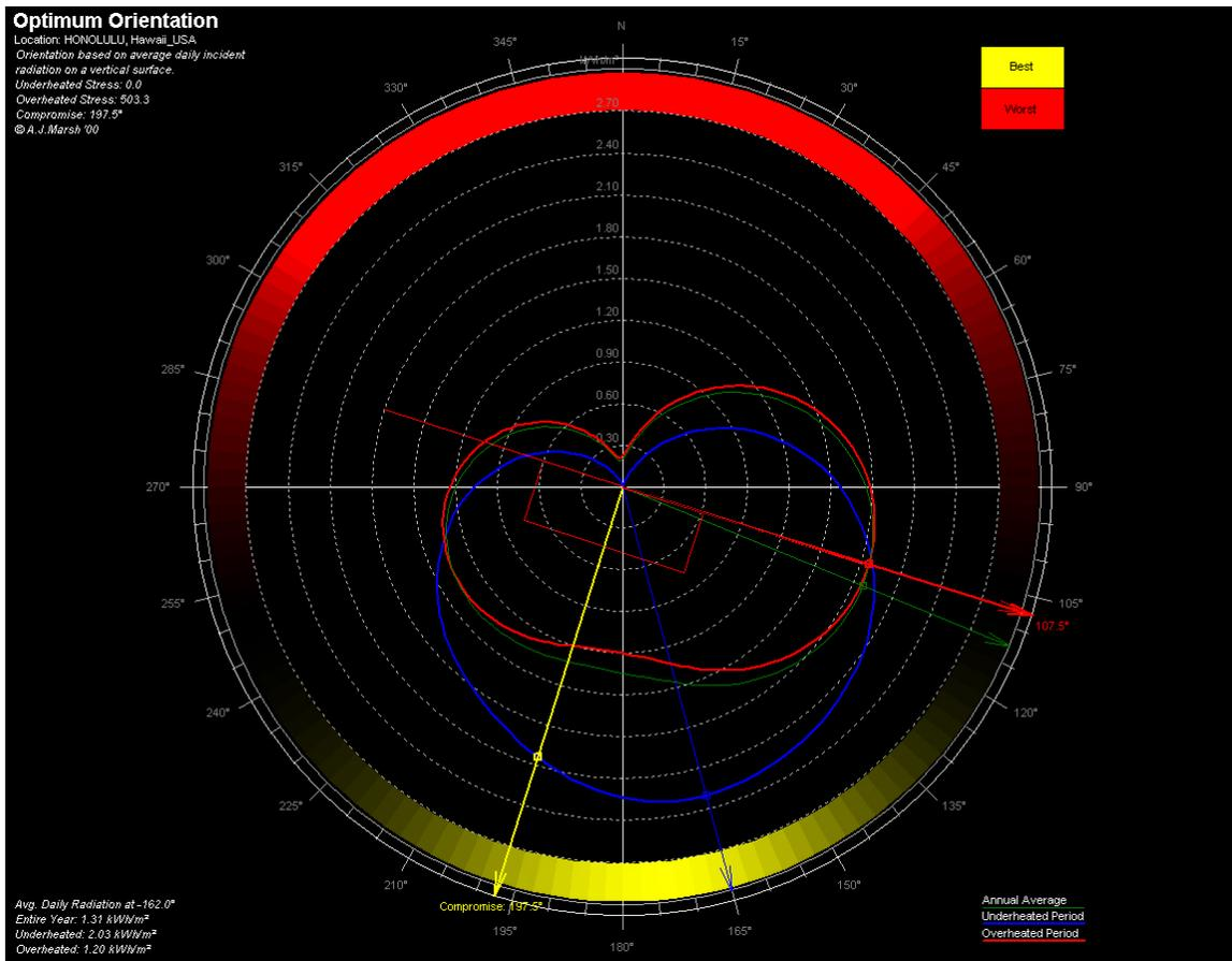
Fig. 36 – Optimum Building Orientation for Honolulu, Hi, for Solar Gains Mitigation.
