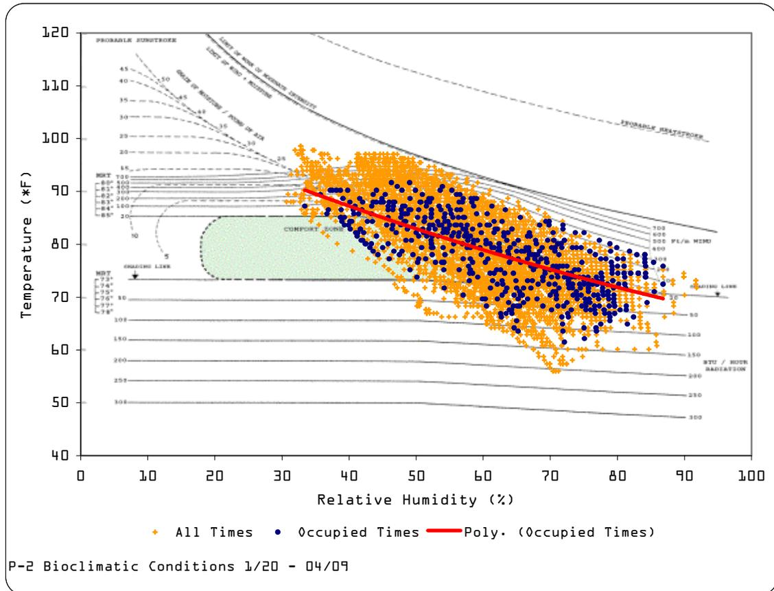
Fig. 20 - Bioclimatic Chart of P-2 from 01/20/03 to 04/09/03.
