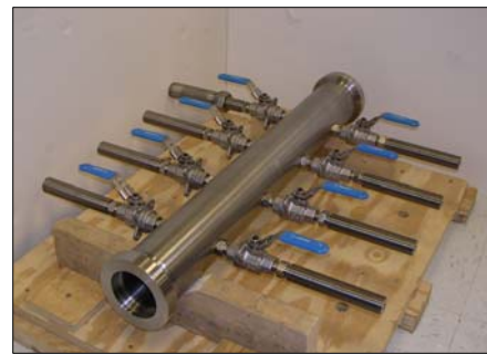
The IPTC is used to measure geophysical and mechanical properties of hydrate bearing cores under in situ pressures (Ga. Tech/Chevron JIP)
