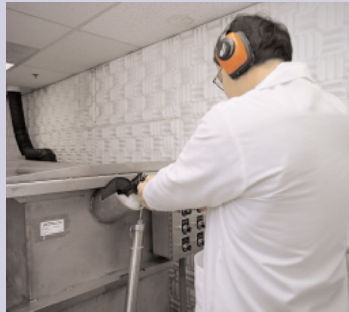
Firearms Specialist firing a weapon into a water tank to recover a bullet and identify its resulting markings.
