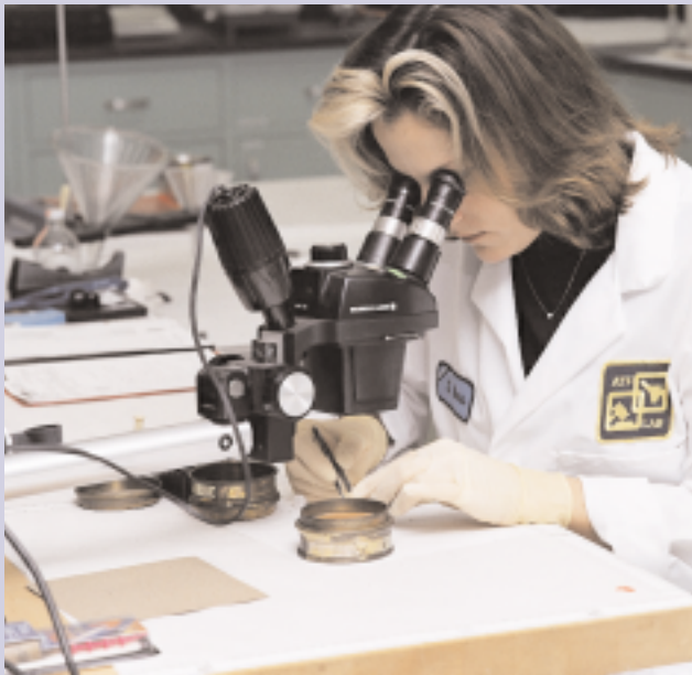
Forensic Chemist examining sifted debris from a bombing for intact explosives and component parts.
